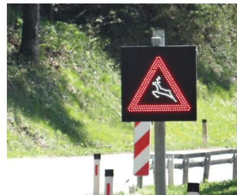
Dynamic traffic sign, which alerts drivers to wildlife near the road.
