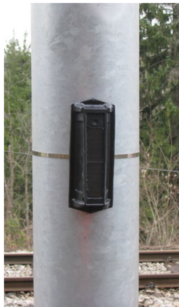
Acoustic deterrents were installed on electric poles along the railway tracks in Slovenia to reduce train-bear collisions.
