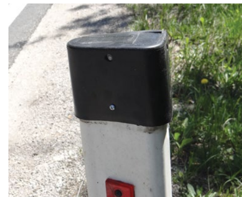
Acoustic deterrents with sensors were installed into the roadside traffic pillars on most critical road sections.
