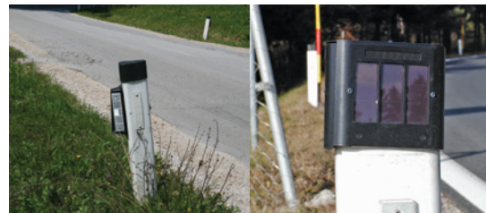
Two types of acoustic deterrent that have been used so far in Slovenia.
