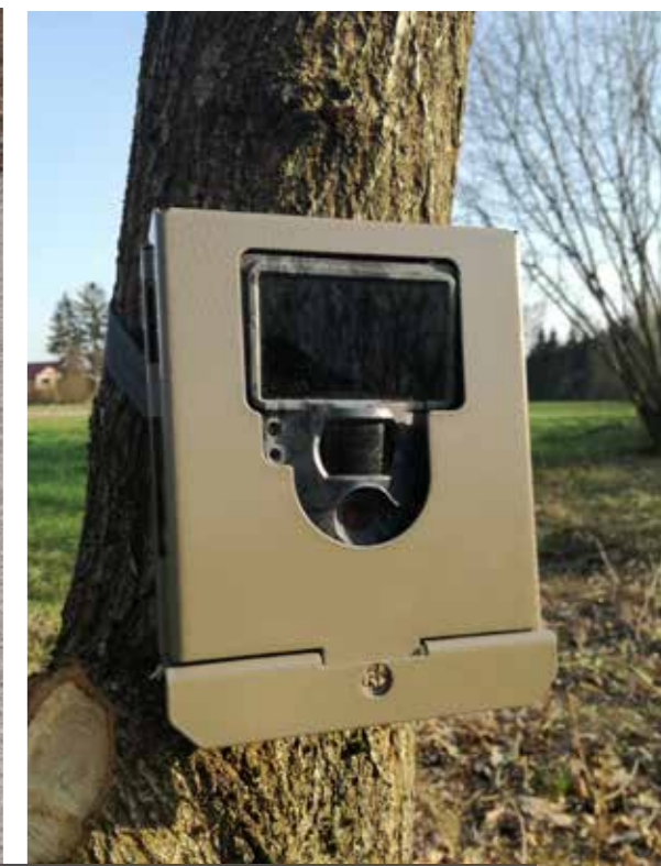
Bear tracks on sand beds (left) used to monitor effectiveness of crossing structures. Modern camera traps (right) can detect animal passing during day as well as nighttime using 940 nm IR light which is invisible for mammals. (Potočnik H.)
