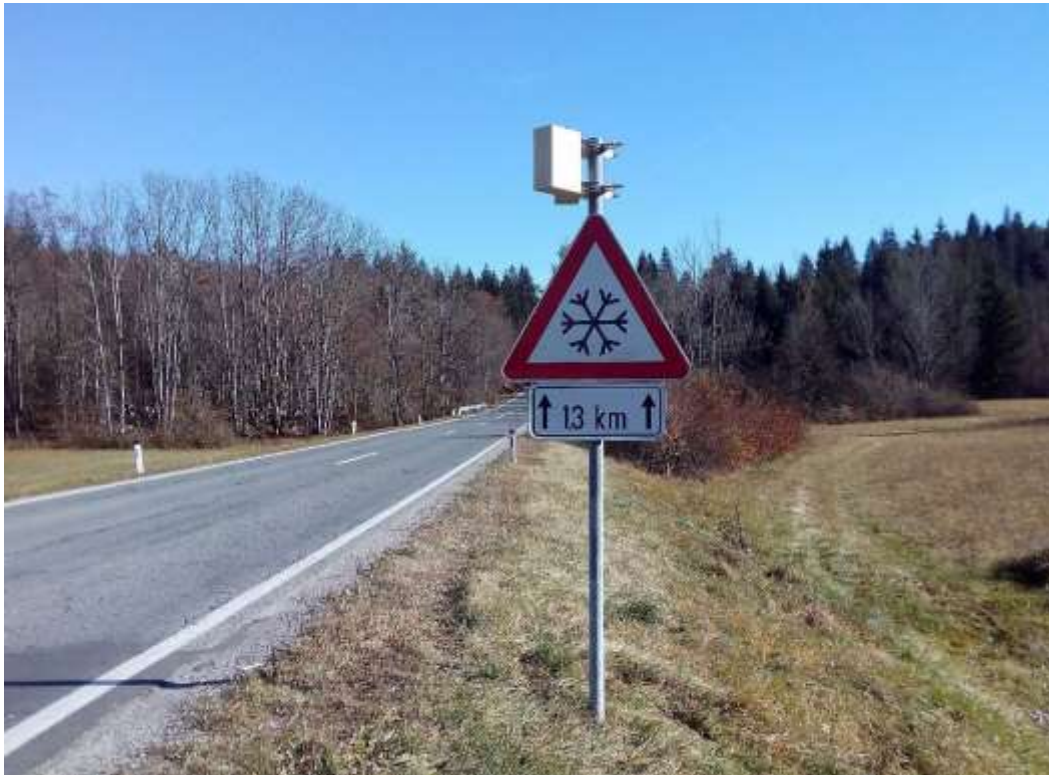
Figure 19: Traffic counter placed on the pole of traffic sign near Dolenja vas (Jasnica).
