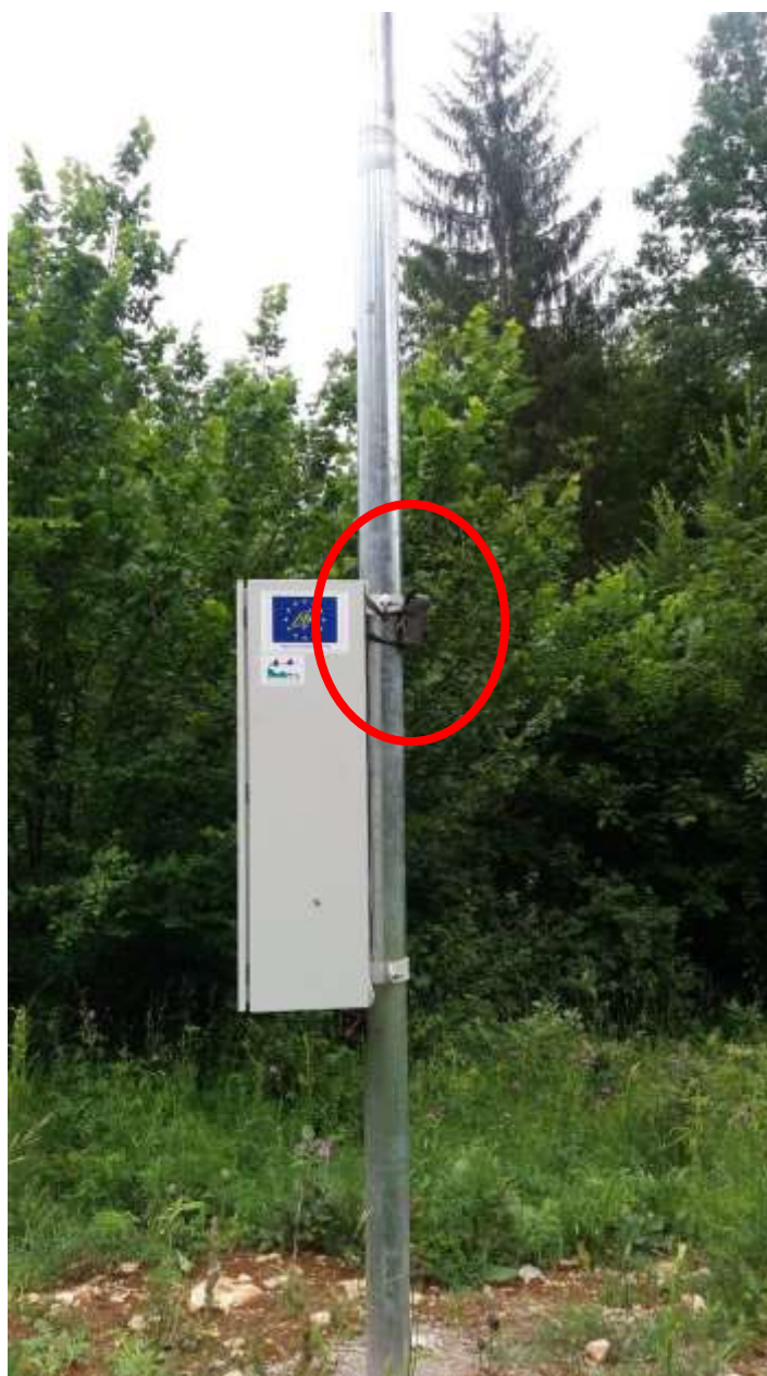
Figure 49: Installation of IR camera at Turjak, near the road Ljubljana – Kočevje; location where animals, that want to cross the road at this section, usually pas (photo: I. Jelenko Turinek, 2018).
