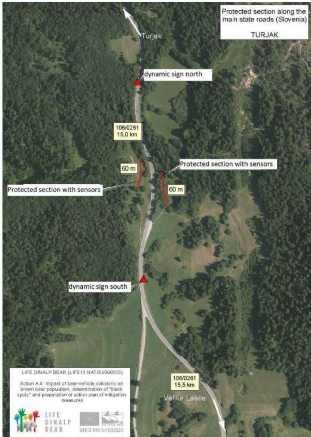
Figure 4: Dynamic traffic sign at Turjak - sensors (red line) and traffic signs (triangle).
