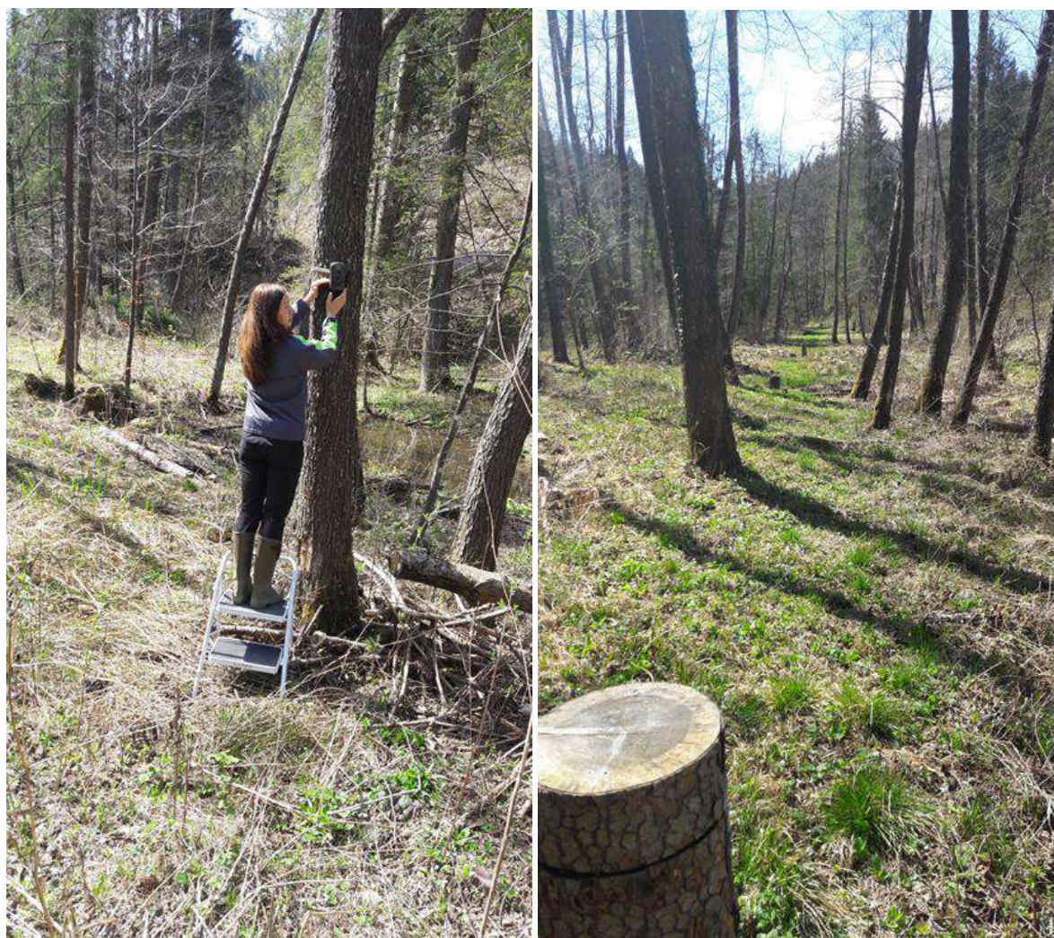
Figure 31: Installation of IR cameras at Ortnek and sensors in wooden stumps capable to detect large animals approaching the roadway (photo: Z. Pavšek, 2017).
