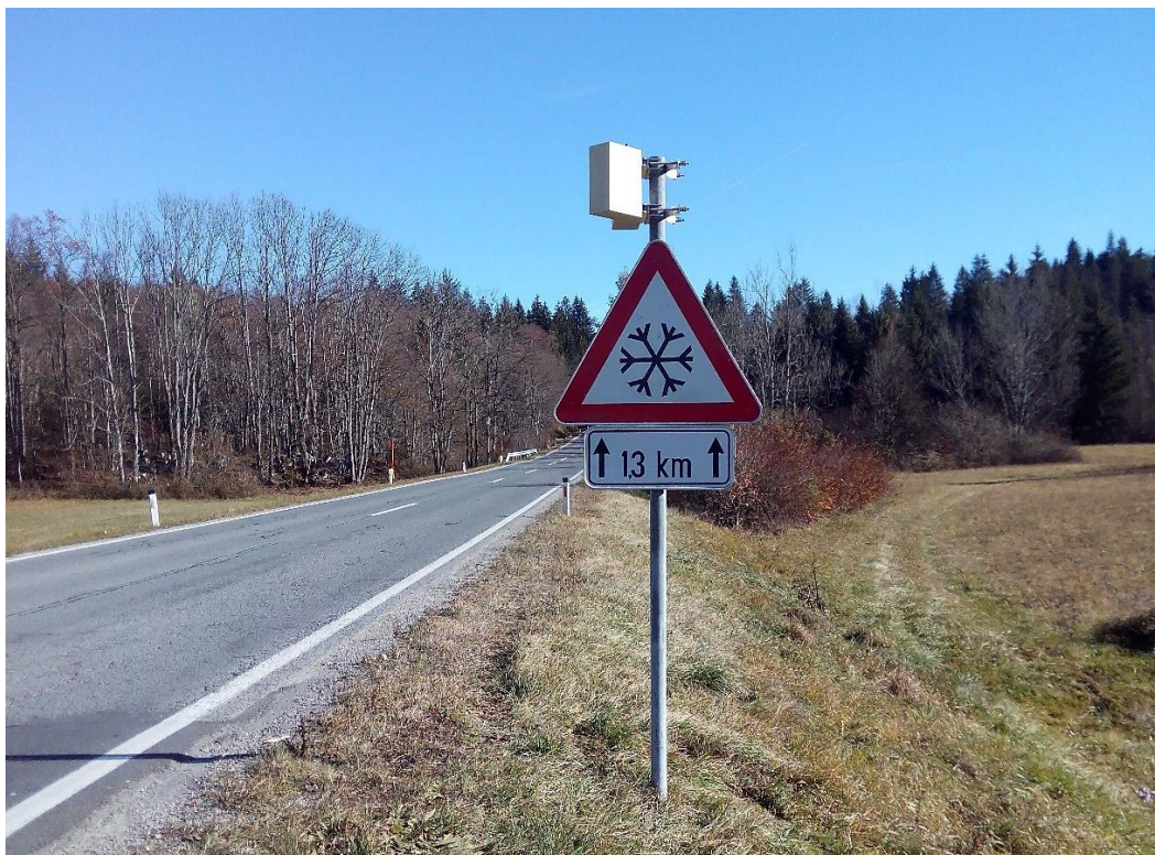
Figure 16: Traffic counter placed on the pole of traffic sign near Dolenja vas (Jasnica).
